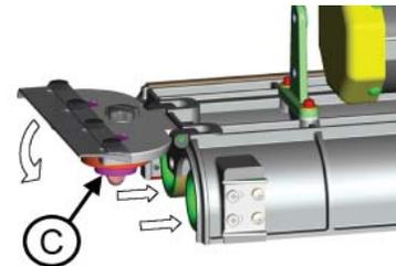
3. Insert **Idle Hubs (C)** into the brushes while closing the hinged cover. Tighten the knob on the cover by hand, ensuring that the hinged idle cover is flush to the deck.
