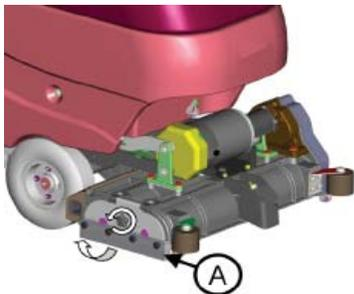
1. Raise brush deck. Unscrew the knob on the right side of the deck as shown above. Pull open the **Hinged Cover (A)**.
