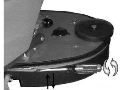
1. Brush Deck may be tilted up for easier brush installation/removal & to clear steep ramps. Lift the handle on the upper lever which connects the brush deck to the machine, tilt the deck up, release the handle & the lever will lock into place. Lift the handle again to move the deck back to horizontal.
