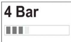
The battery charge level has fallen below the Battery Lockout level and the controller is inhibiting certain machine functions. Charge the battery.
